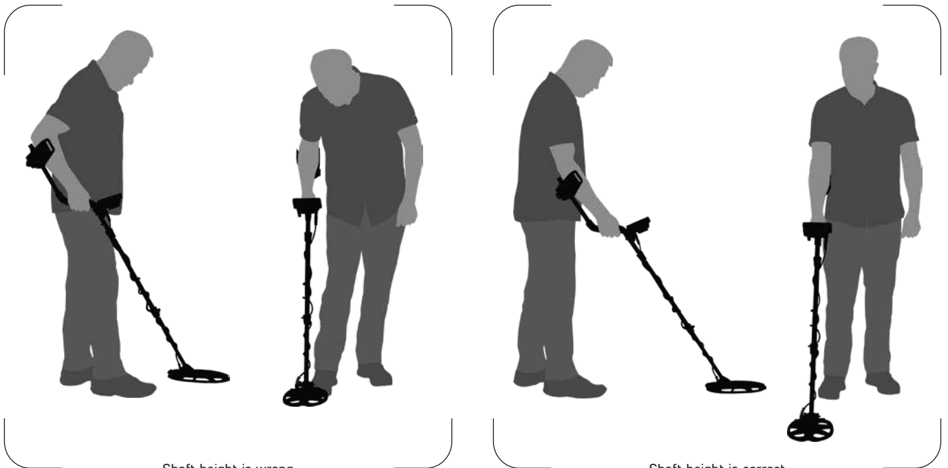
Shaft height is wrong
