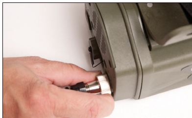
Hand-tighten connector collar.
