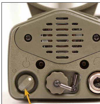
On/Off Switch (shown in On position)
