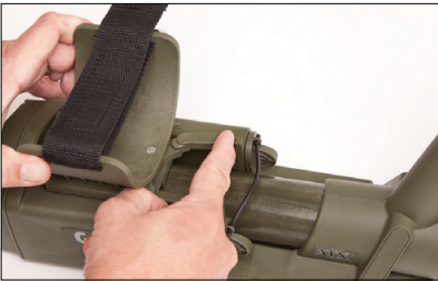
Armrest locking lever shown in open position.
